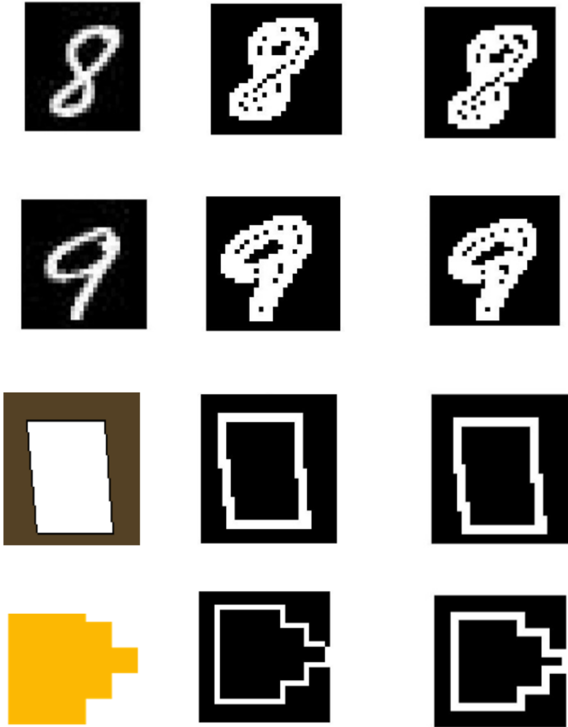
Figure 4.6: Simulation Results: Original Image (Left), Edge Detected Image through MATLAB (Middle), Edge Detected Image through Our Proposed Work (Right)
